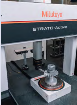
STRATO-Active with rotary table MRT320
