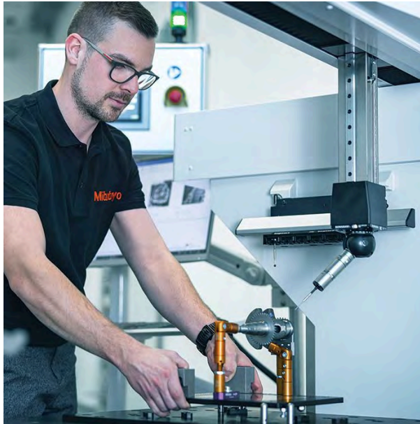
3-point repositioning Pallet Receiver System PRS
