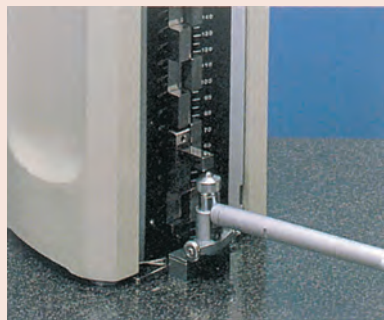
Bore Gauge Series 511 reference setting
