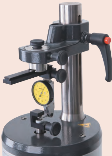
Calibration of Dial Test Indicator (Lever Type) with optional accessories
