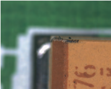
Normal microscope observation (upper) With a height difference, only the upper or lower plane can be focused.
