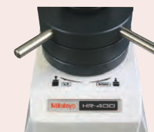
HR-400 Automatic preliminary test force brake
