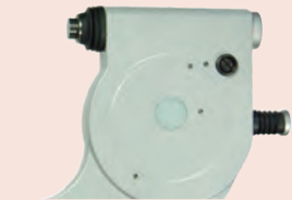
Adjusting screw for dial comparator \pm 5 \mu m
